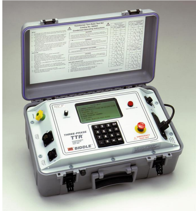
FIG 6. Transformer Turns Ratio Meter Unit from Megger Company, model TTR.
