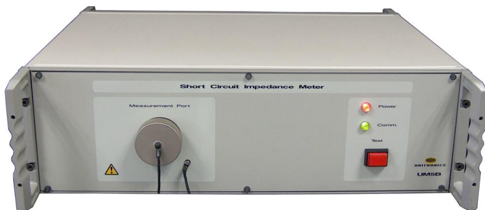
FIG 7. 3phase short circuit impedance unit from UNITRONICS company, model UM5B.
