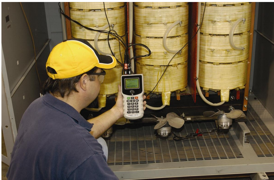
FIG 3. Monophase transformer turns ratio unit, from Megger Company, model TTR100.
