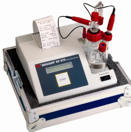
FIG 25. System for moisture determination in oil, from Megger, Model KF875.
