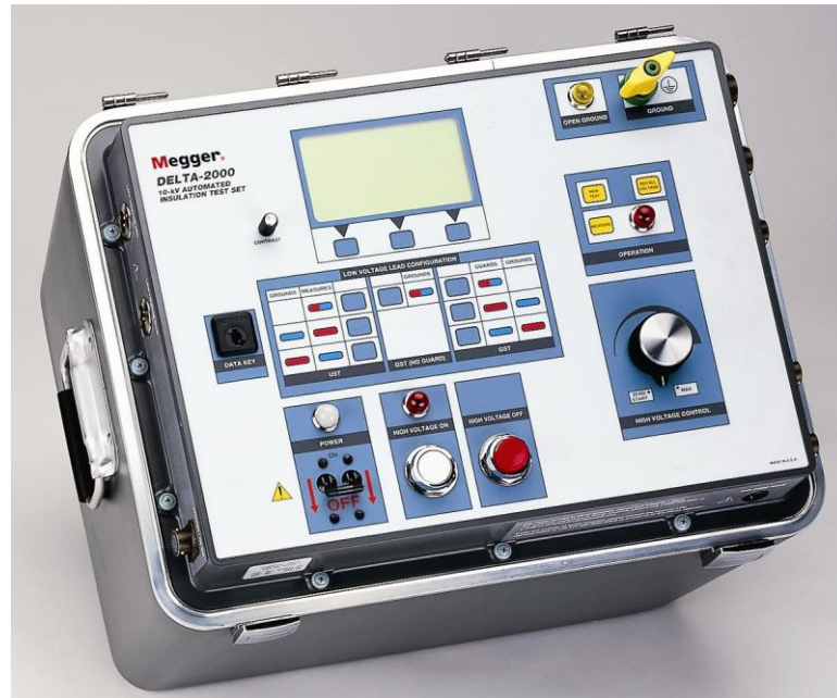
FIG 23. Tan delta meter from Megger, model Delta 2000.
