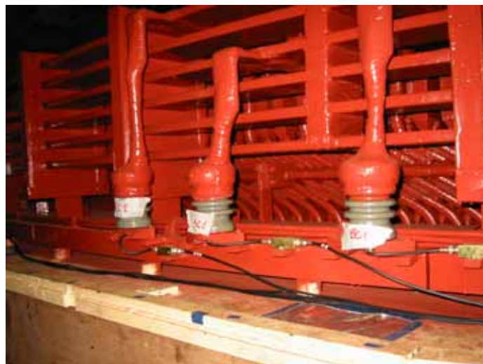
Fig. 2. Usual connection of hydro capacitive couplers.
