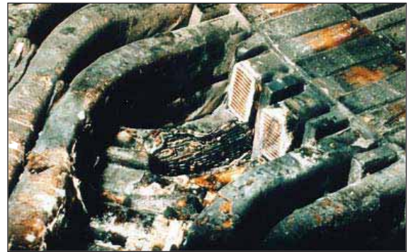
Stator Winding Failure
