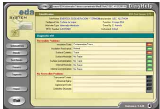
Figure 9 DiagHelp software shows contamination.
