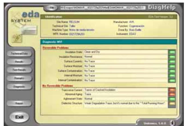
Figure 10 The same machine diagnosed after cleaning.
