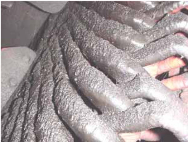
Figure 6 Example of contamination with oil detected with EDA system.
